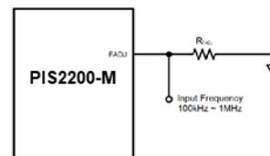
Figure 2. Clock Synchronization
