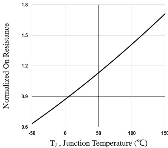
**Fig.2 Normalized RD<sub>SON</sub> vs.  $T_J$**
