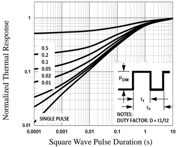
**Fig.8 Normalized Transient Impedance**
