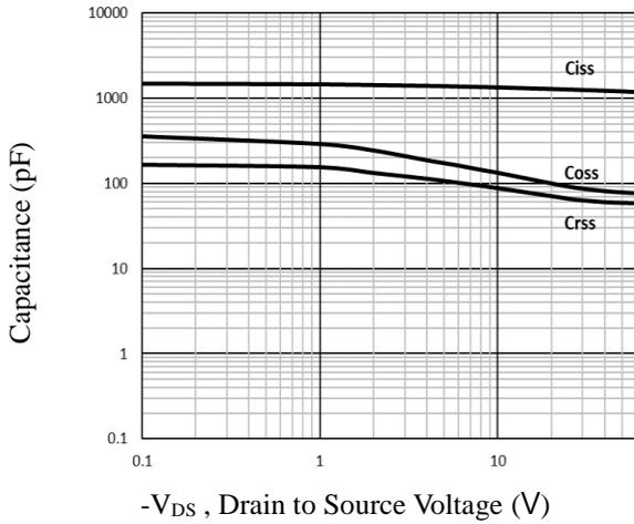
**Fig.7 Capacitance Characteristics**
