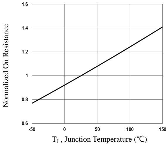
**Fig.2 Normalized RD<sub>SON</sub> vs.  $T_J$**
