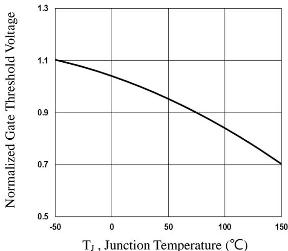
**Fig.3 Normalized V<sub>th</sub> vs. T<sub>j</sub>**
