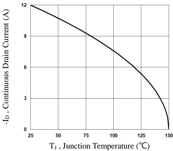
**Fig.1 Continuous Drain Current vs. T<sub>c</sub>**
