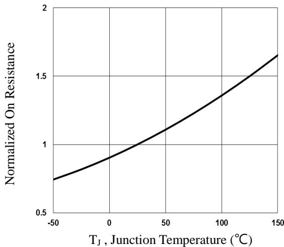
**Fig.2 Normalized RDSON vs. T<sub>c</sub>**
